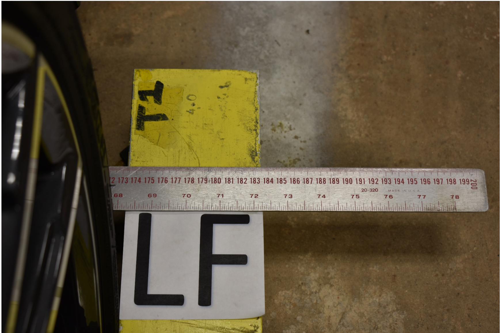
FIGURE 5.17 FRONT LEFT TIRE REAR MEASUREMENT
